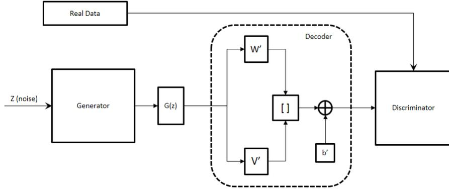
Fig. 2: Block diagram GAN training module.
