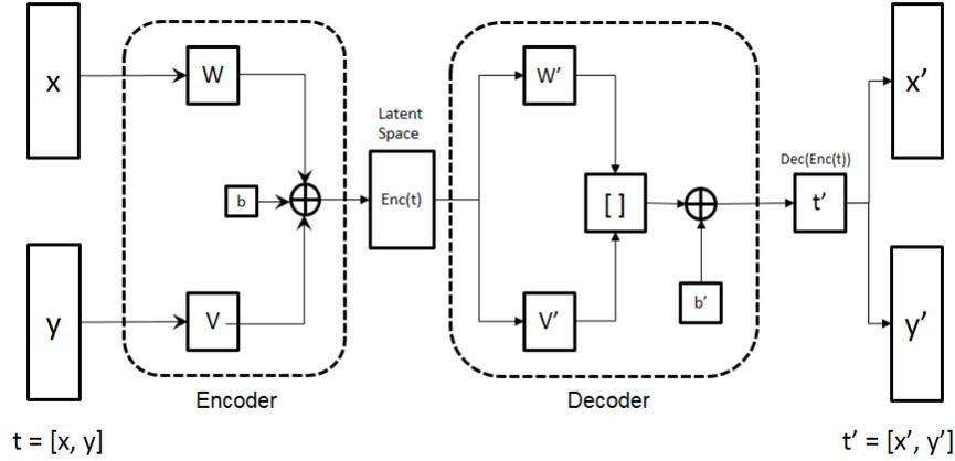
Fig. 1: Block diagram of Correlational Neural Network
